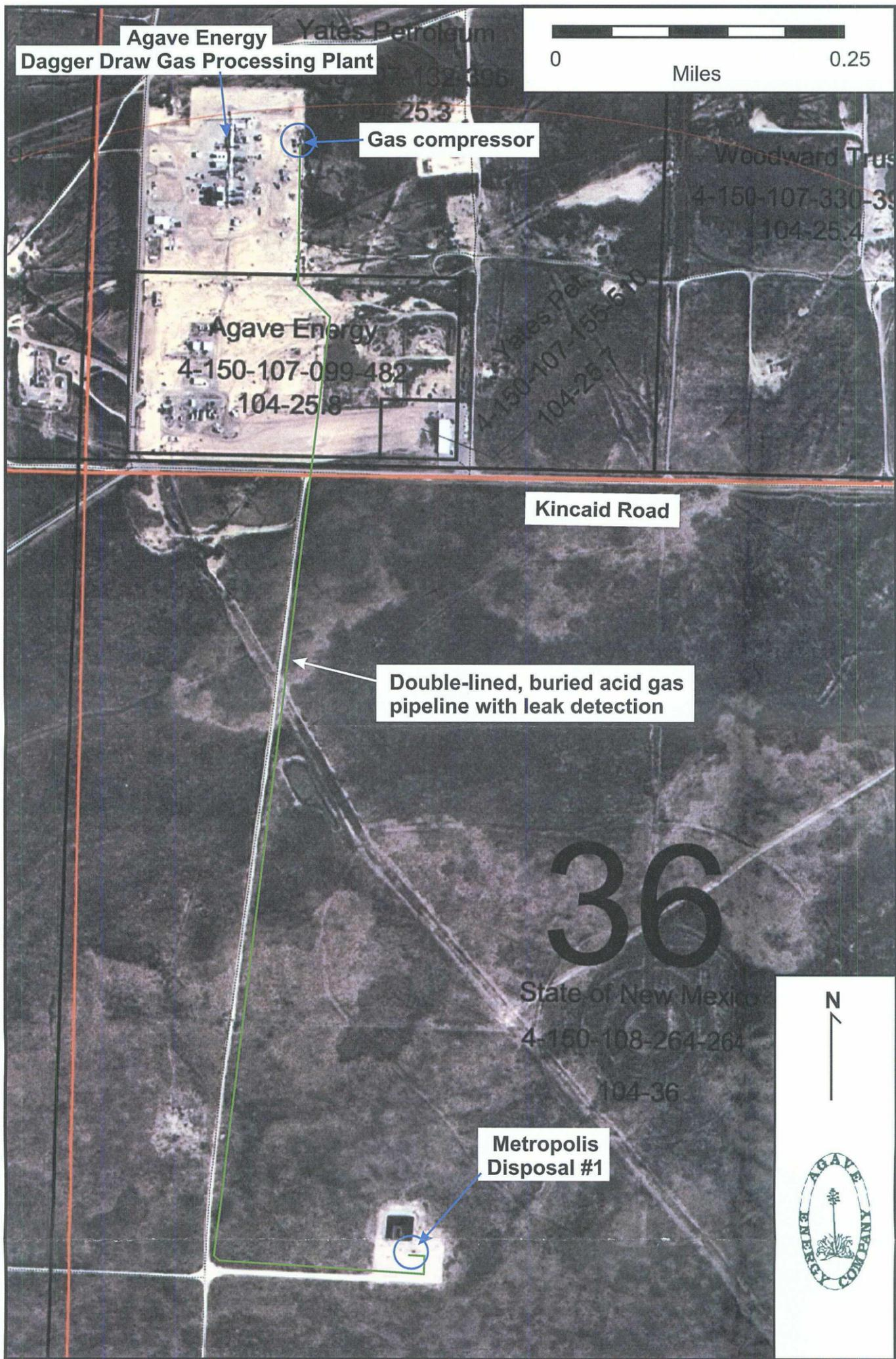
Map 2: General Diagram of Agave Dagger Draw Gas Plant and Location of Pipeline Connecting the Plant with the Metropolis Disposal #1 Well. Please note that the former Agave Energy Facility located immediately south of the Dagger Draw Gas Processing Plant is an inactive, unmanned facility.
