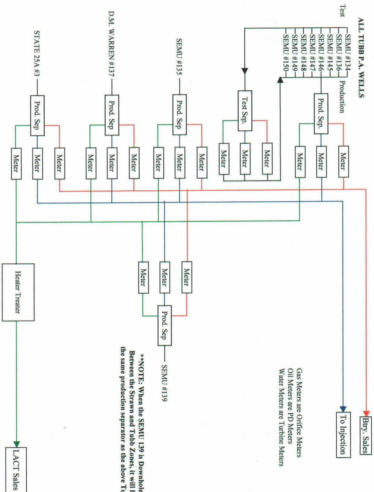
**\*\*NOTE:** When the SEMUR 139 is Downhole Commingling Between the Strawn and Tubb Zones, it will be moved into the same production separator as the above Tubb P.A. Wells.
