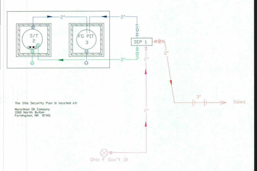
Draining Phaser Sales valve closedl Drain valves sealed open! Fill valve sealed closed! Equalizer valve sealed closed! Sales Phasei Sales valve open! Drain valves sealed closed! Fill valve sealed closed! Equalizer valve sealed closed! Production Phase: Sales valve closed! Drain valve sealed closed! Fill valve open! Equalizer valve open! - VATER
