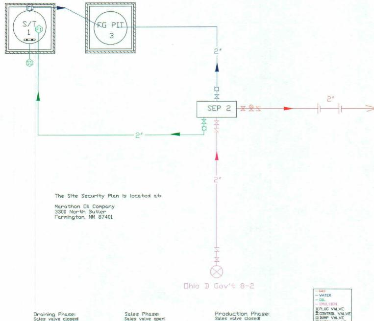
Draining Phase: Sales valve closed! Drain valves sealed open! Fill valve sealed closed! Equalizer valve sealed closed!
