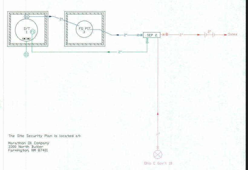
Draining Phase: Sales valve closed! Drain valves sealed open! Fill valve sealed closed! Equalizer valve sealed closed!
