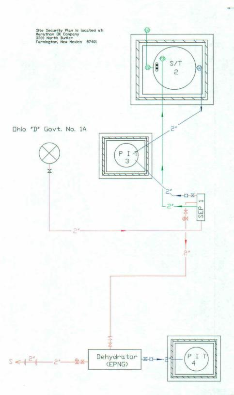
Sales Phase: Sales valve open! Drain valves sealed closed! Fill valve sealed closed! Equalizer valve sealed closed! Production Phase: Sales valve closed! Drain valve sealed closed! Fill valve open! Equalizer valve open! Draining Phase: Sales valve closed! Drain valve sealed open! Fill valve closed! Equalizer valve closed!
