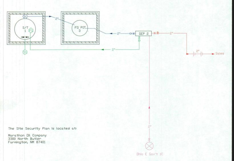
Draining Phase: Sales valve closed! Drain valves sealed open! Fill valve sealed closed! Equalizer valve sealed closed! Sales Phase: Sales valve open! Drain valves sealed closed! Fill valve sealed closed! Equalizer valve sealed closed! Production Phase: Sales valve closed! Drain valve sealed closed! Fill valve open! Equalizer valve open! - DIL
