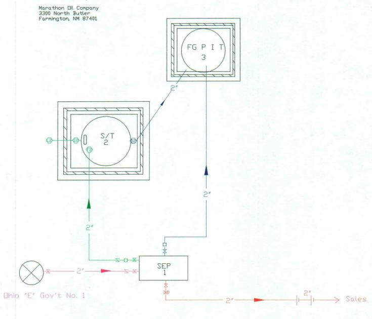
Draining Phase: Sales valve closed! Drain valves sealed open! Fill valve sealed closed! Equalizer valve sealed closed! Sales Phase: Sales valve open! Drain valves sealed closed! Fill valve sealed closed! Equalizer valve sealed closed!
