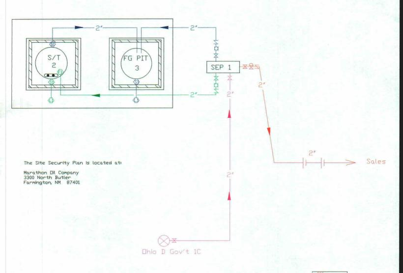
Draining Phasei Sales valve closed! Drain valves sealed open! Fill valve sealed closed! Equalizer valve sealed closed! Sales Phase: Sales valve open! Drain valves sealed closed! Fill valve sealed closed! Equalizer valve sealed closed! Production Phase: Sales valve closed! Drain valve sealed closed! Fill valve open! Equalizer valve open! - WATER
