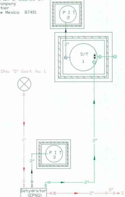
Sales Phasei Sales valve open! Drain valves sealed closed! Fill valve sealed closed! Equalizer valve sealed closed!
