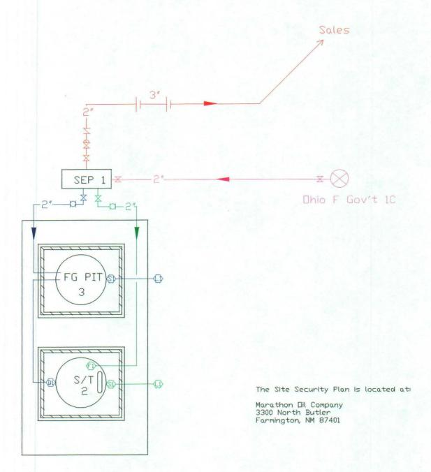
Draining Phase: Sales valve closed! Drain valves sealed open! Fill valve sealed closed! Equalizer valve sealed closed! Sales Phase: Sales valve open! Drain valves sealed closed! Fill valve sealed closed! Equalizer valve sealed closed!
