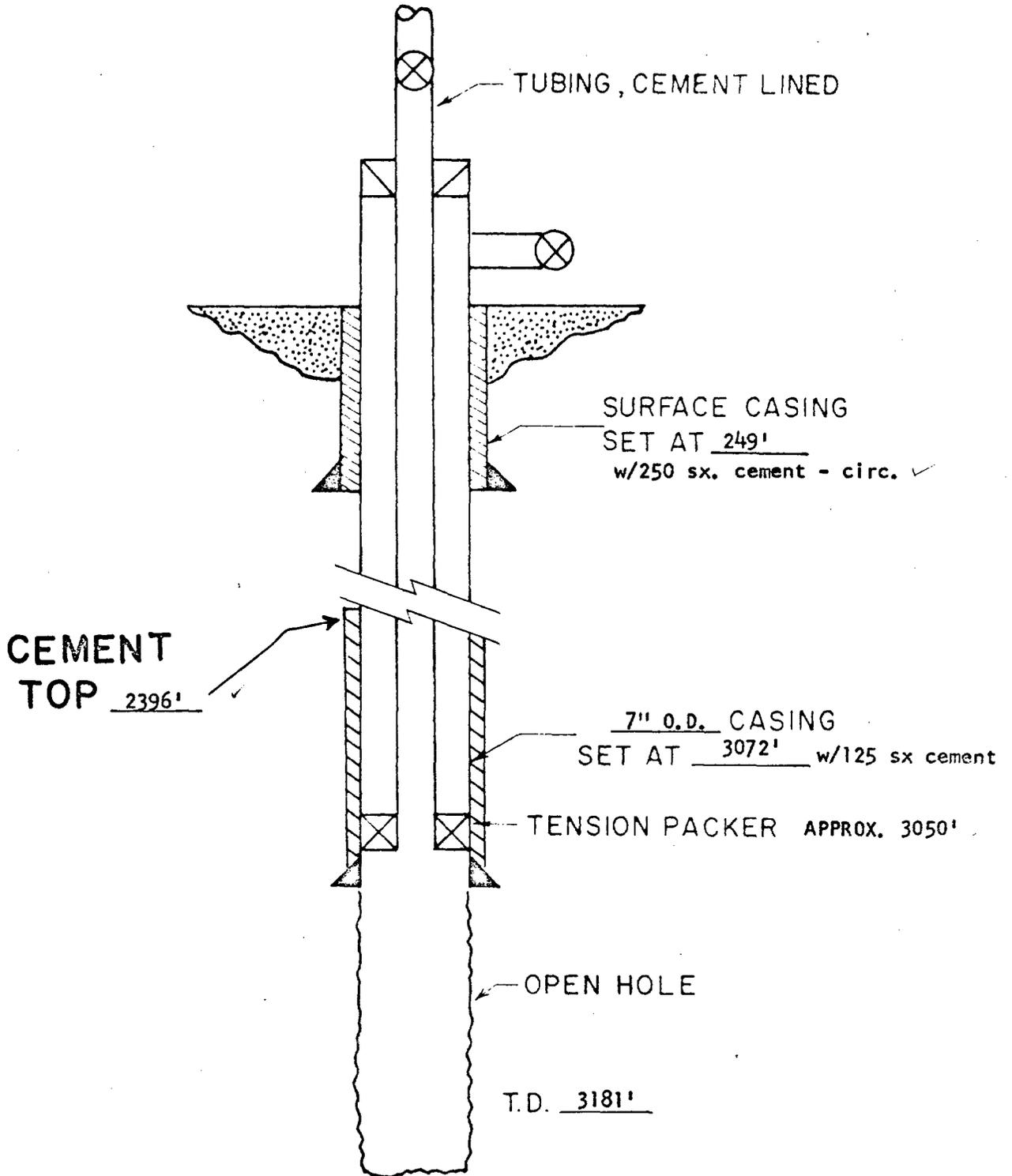
WATER INJECTION WELL SCHEMATIC
