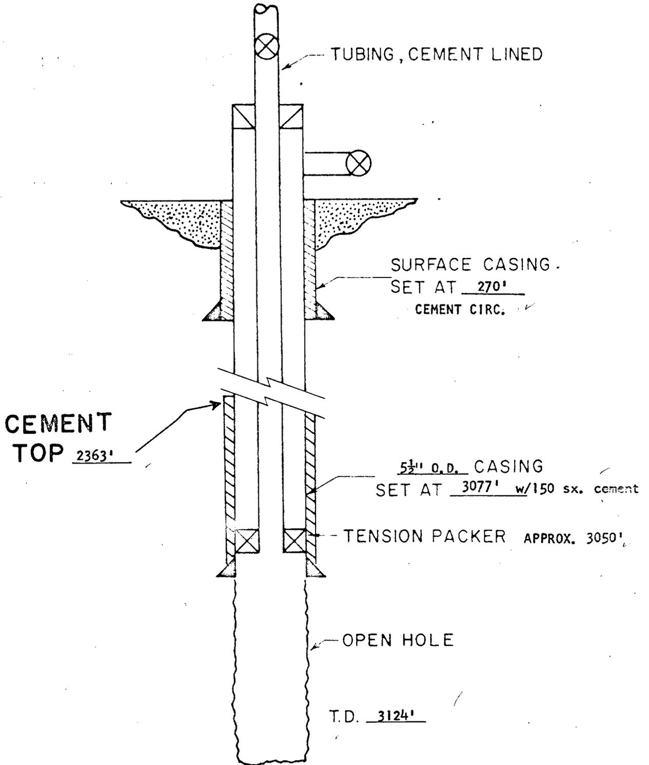
WATER INJECTION WELL SCHEMATIC
