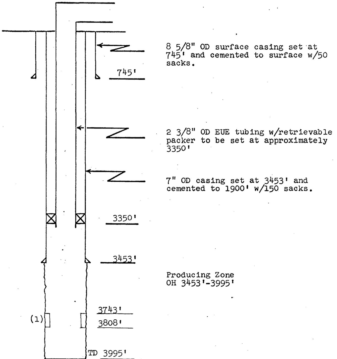
(1) 5 1/2" OD liner from 3743'-3808' cemented w/12 sacks Calseal - liner was perforated 3743'-3808'.
