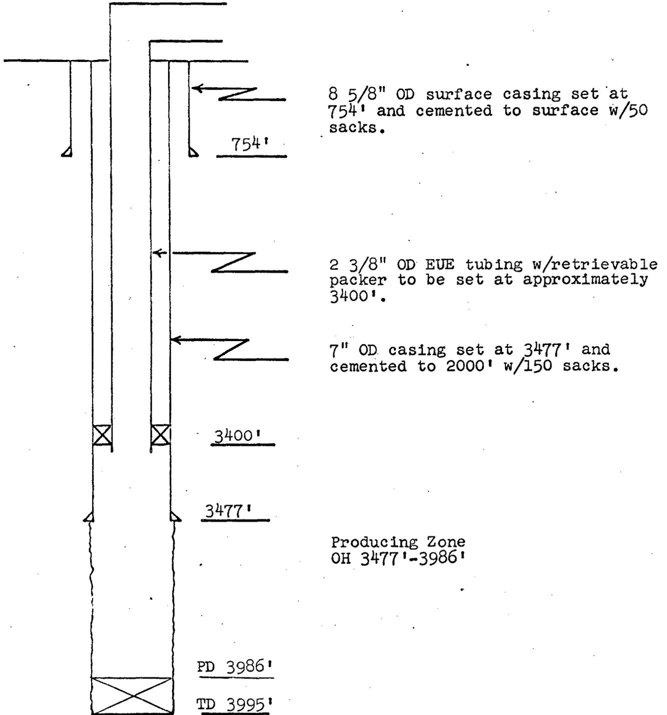
8 5/8" OD surface casing set at 754' and cemented to surface w/50 sacks.
