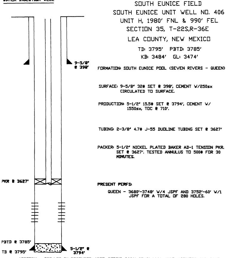
HISTORY - DRILLED IN DECEMBER, 1957. PERF'D 3680'-3748' W/4 JSPF. ACIDIZED AND SAND FRAC W/10,000# OF SAND. IP - 180 BOPD, 0 BWPD & 152 MCFD. TA'D IN 1965. IN MARCH, 1975 INSTALLED ROD PUMP. IN FEBRUARY 1976 - PERF 3752'-3760' W/1 JSPF. ACIDIZED AND SAND FRAC W/20,000# OF SAND. 12/91 - ACIDIZE W/4000 GAL 15% NEFE ACID. SAND FRAC W/16,000 GAL OF GELLED FLUID CONTAINING 34,000# OF 20/40 SAND W/1-6 PPG, AIR 20 BPM. SHUT-IN OIL WELL. AWAITING PERMIT FOR INJECTION.
