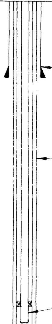
8 5/8" CASING SET @ 354' CEMENTED WITH 165 SACKS. CIRCULATED.
