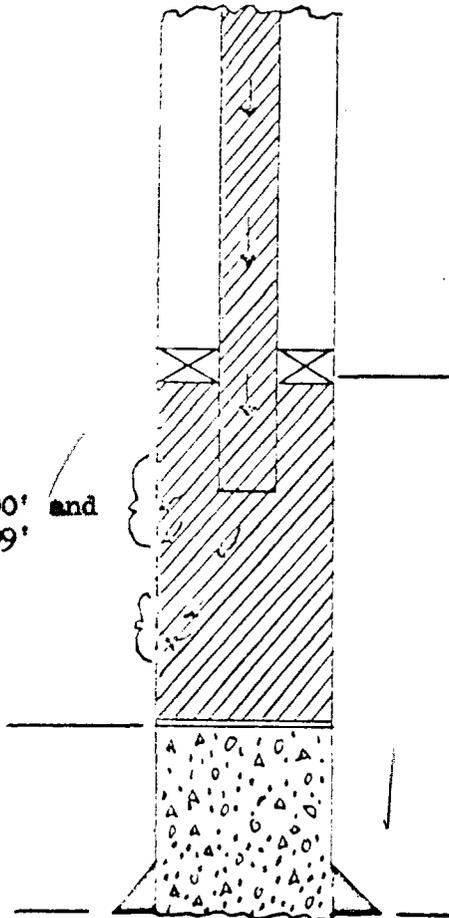
5-1/2" O.D., J-55, 14# Casing set at 1360'. Cemented with 110 Sacks.
