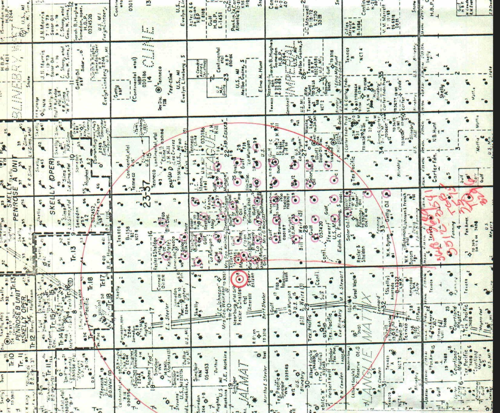
**PLAT SHOWING LOCATION OF RESLER AND SHELDON SALT WATER DISPOSAL WELL #1, AND THE LOCATION OF ALL OTHER WELLS WITHIN A RADIUS OF TWO MILES.**
