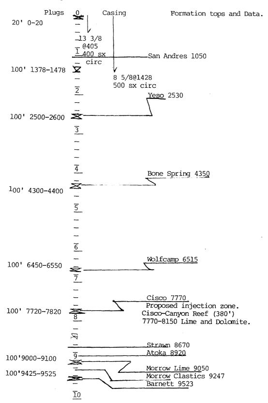
XII I have examined available geologic and engineering data and find no evidence of open faults or any other hydrologic connection between the disposal zone and any underground source of drinking water.
