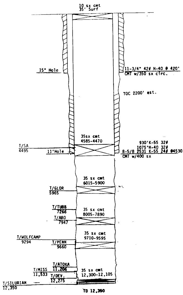
Tubing size 2-3/8 lined with AMF TK75 (material) set in aBaker 'AD-1' Tension (brand and model) packer at 4300 feet
