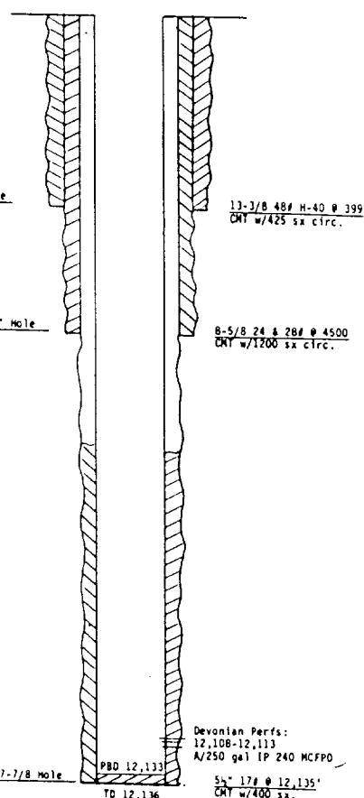
Surface CasingSize 13-3/8, Cmtd w/425 sx.TOC Circ ft. as per drilling rpt.Hole size 17-1/2"Intermediate CasingSize 8-5/8, Cmtd w/400 sx.TOC surf ft. as per drilling reportHole size 12-1/4"Long stringSize 5-1/2, Cmtd w/400 sx.TOC unknown ft. as per \_\_\_\_\_Hole size 7-7/8"Liner NONE
