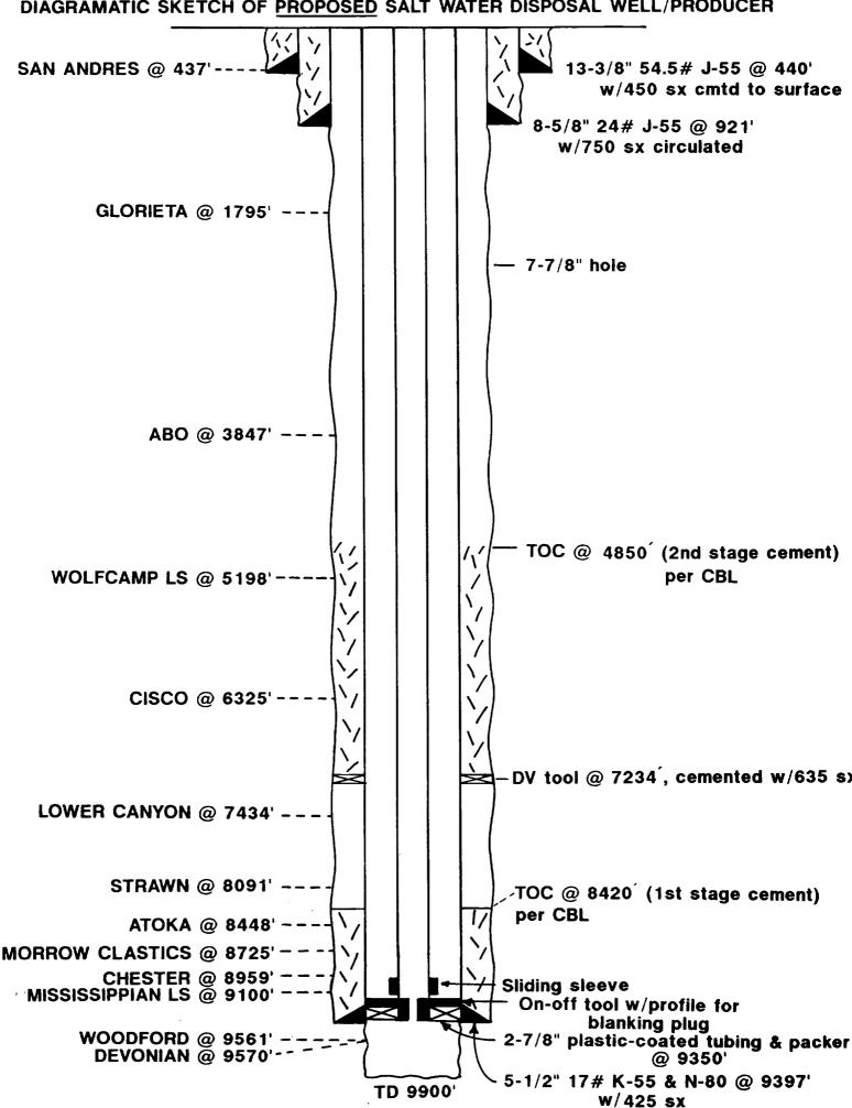
Propose to drill out plug @ 9366' and clean out hole to TD of 9900'. Plan to replace 2-7/8" tubing w/plastic-coated 2-7/8" 6.5# J-55 tubing and Guiberson VI or Baker plastic-coated or nickel-plated packer set @ 9350'. Propose to inject Dagger Draw Upper Pennsylvanian-produced waters down the tubing into the Devonian open hole
