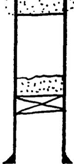
4 1/2" casing set at 9500' with 650 sx of \_\_\_\_\_ cement
