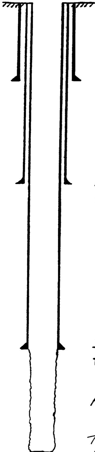
13<sup>3</sup>/<sub>8</sub>" casing set at 395' with 500 sx of \_\_\_\_\_ cement
