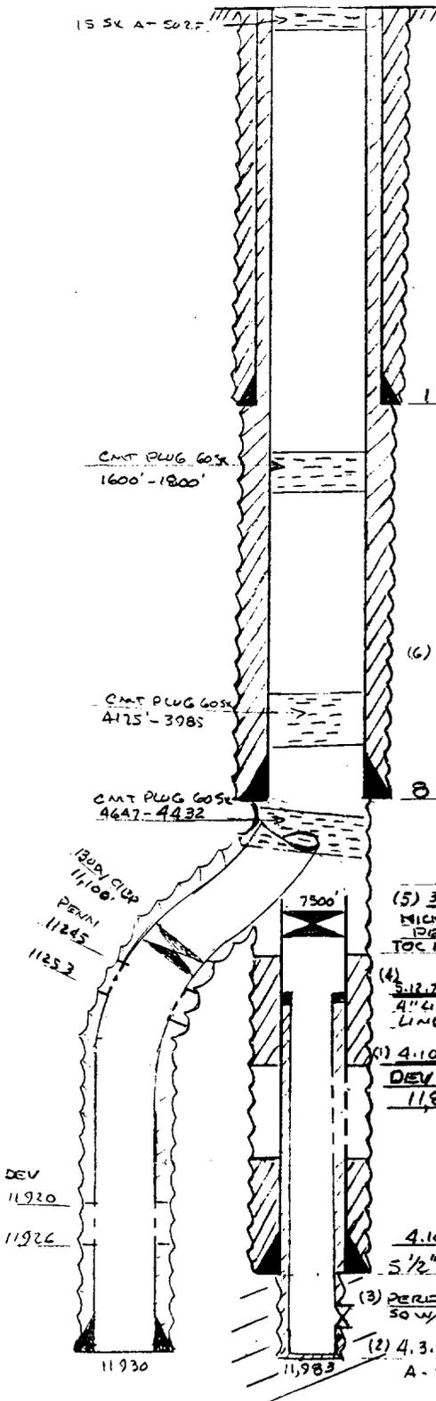
$13\frac{3}{8}$  (43") casing set at 249' with 300 sx of cement.
