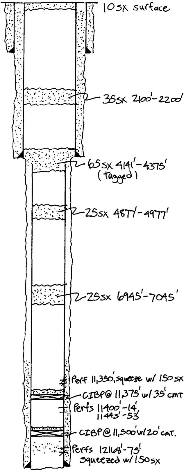
13 3/8" casing set at 235' with 225 sx of cement.
