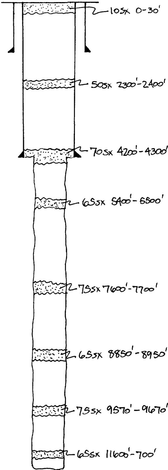
13<sup>3</sup>/<sub>8</sub> " casing set at 260 ' with 365 sx of cement.
