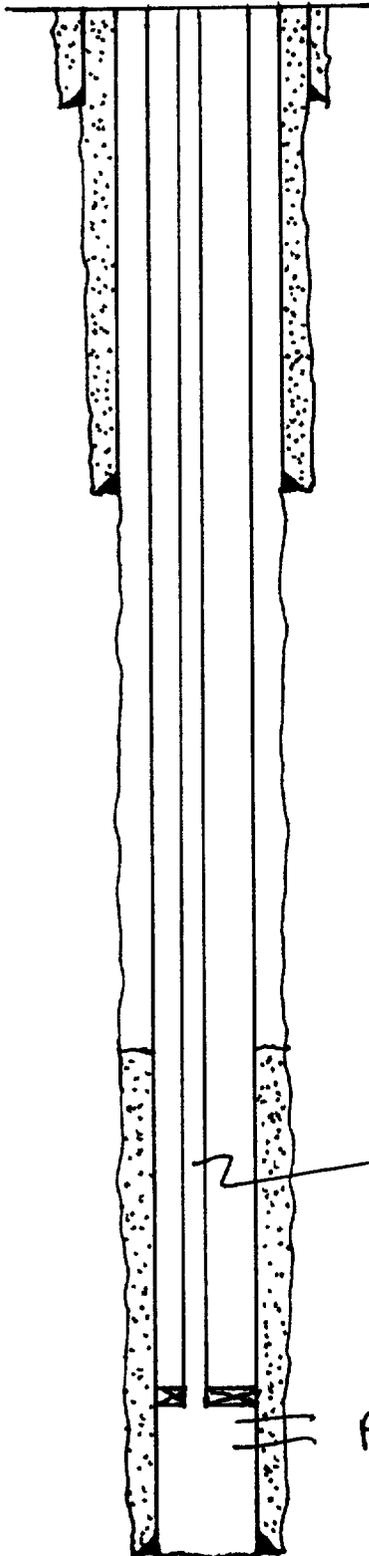
13 3/8 " casing set at 240 ' with 250 sx of cement.
