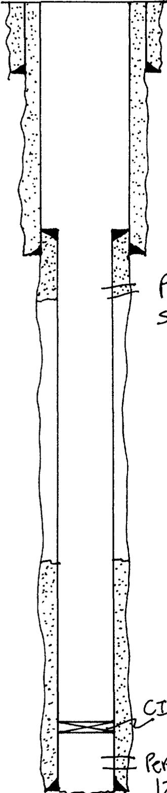
1 3/8 " casing set at 344 ' with 400 sx of cement.
