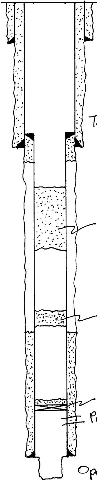
1 1/4 " casing set at 369 ' with 350 sx of cement.
