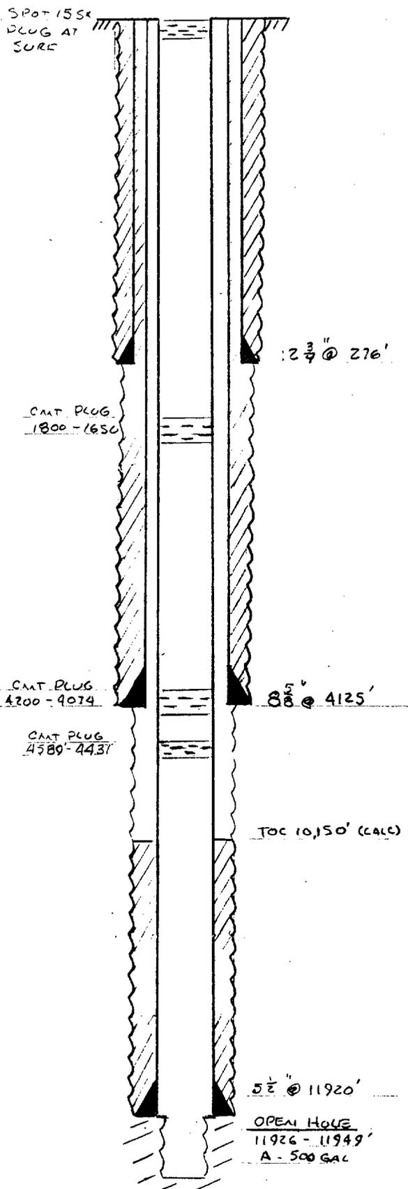
12 <sup>3</sup>/<sub>4</sub> " casing set at 276' with 350 sx of cement.
