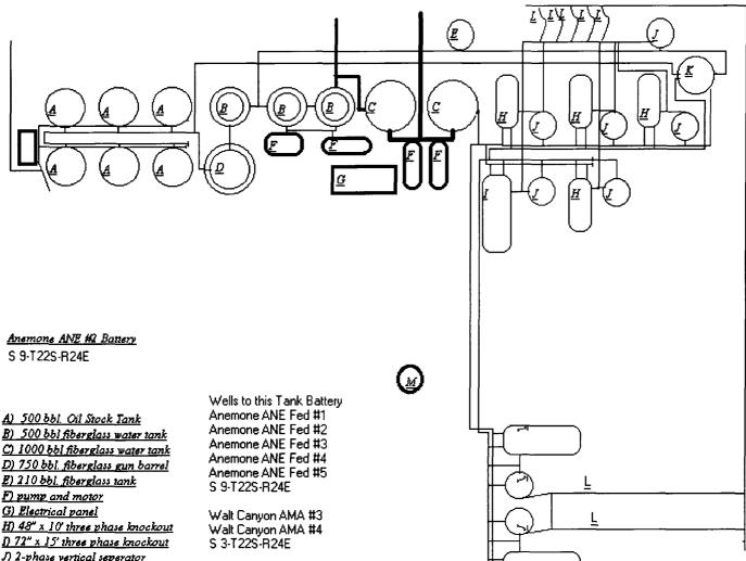
J) 2-phase vertical seperator IQ Heater treater L Gas meter run M) Anemone ANE wellhead N) Lact to Amoco
