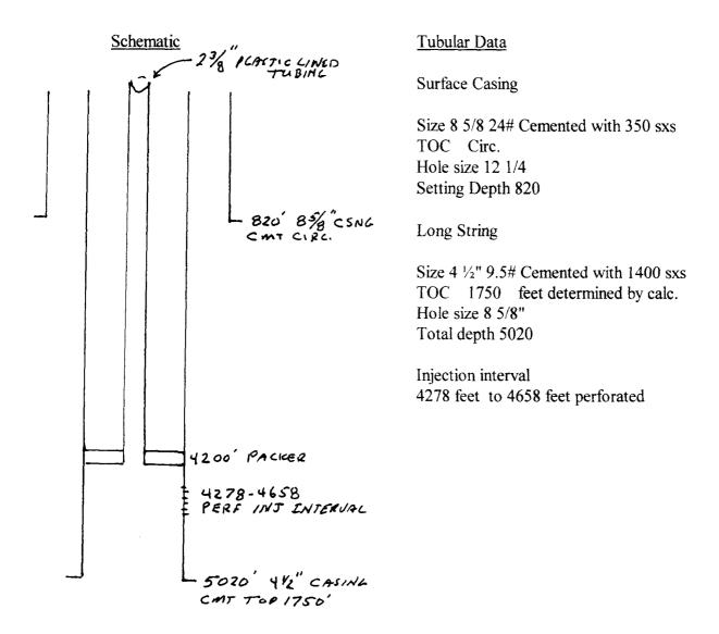
Tubing size 2 3/8" lined with Plastic set in a Baker Loc-set packer at 4200 feet.
