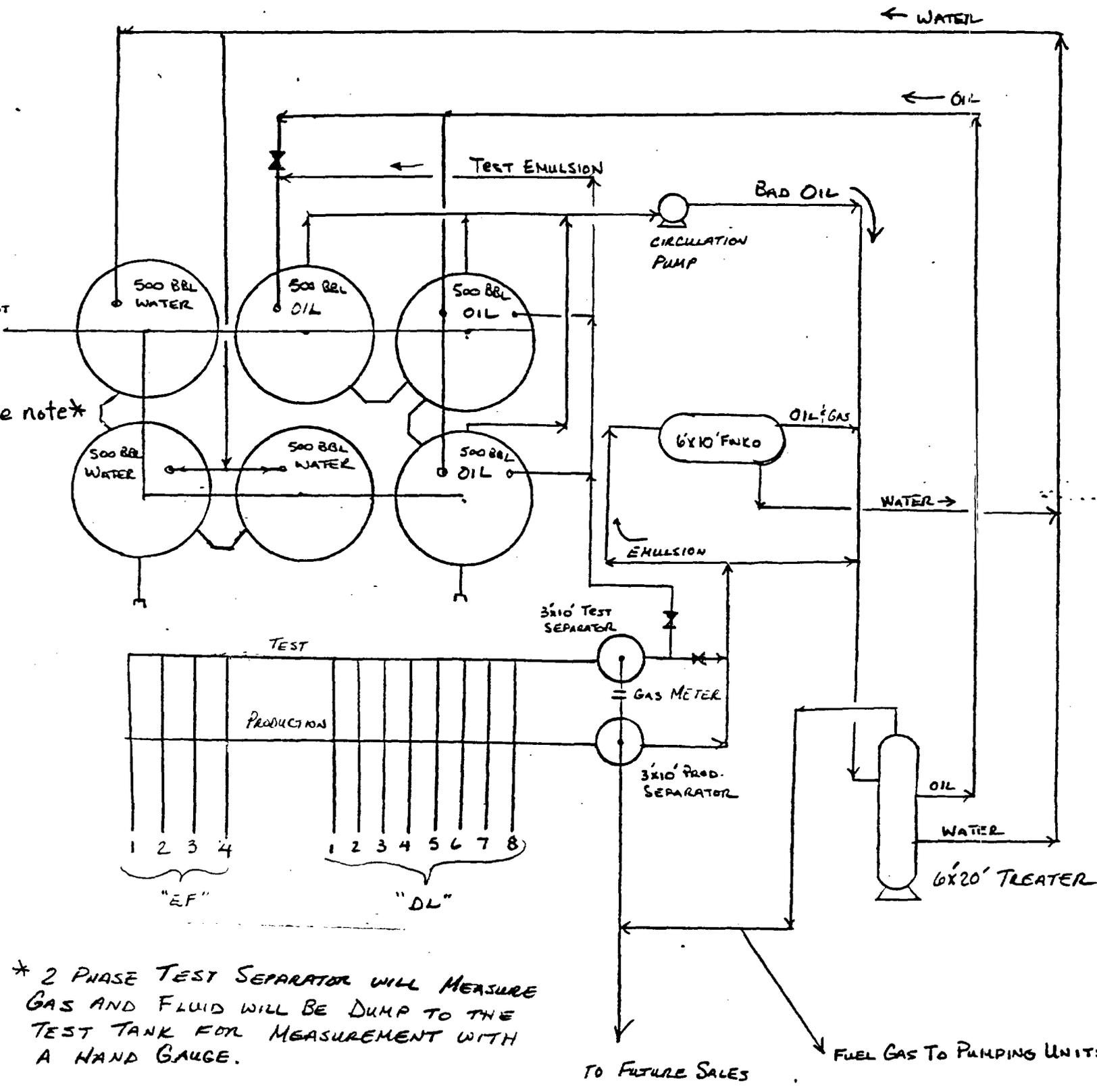
\* 2 PHASE TEST SEPARATOR WILL MEASURE GAS AND FLUID WILL BE DUMP TO THE TEST TANK FOR MEASUREMENT WITH A HAND GAUGE.
