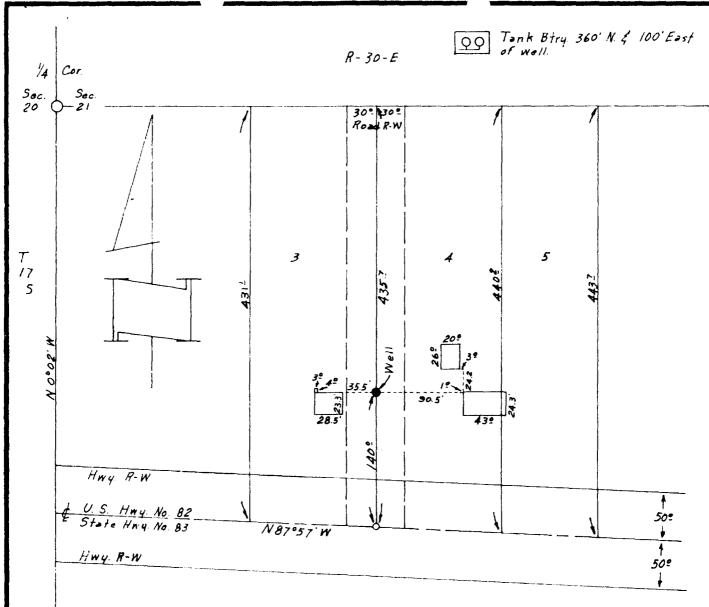
A surveyor's plat showing location of houses, U. S. Highway No. 82 and tank btry. in relation to Franklin, Aston and Fair, Inc., Brigham LC 029342(h) well No. 1-H in the NW NW SW of Section 21, T-17-S, R-30-E, Eddy County, New Mexico.
