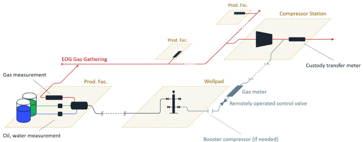
Figure 1 - Closed Loop Gas Capture Schematic
