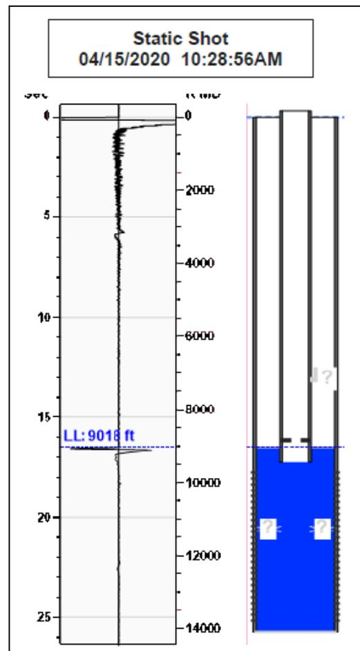
6. 5/6/20 – FL after high rate test (Test #1)
