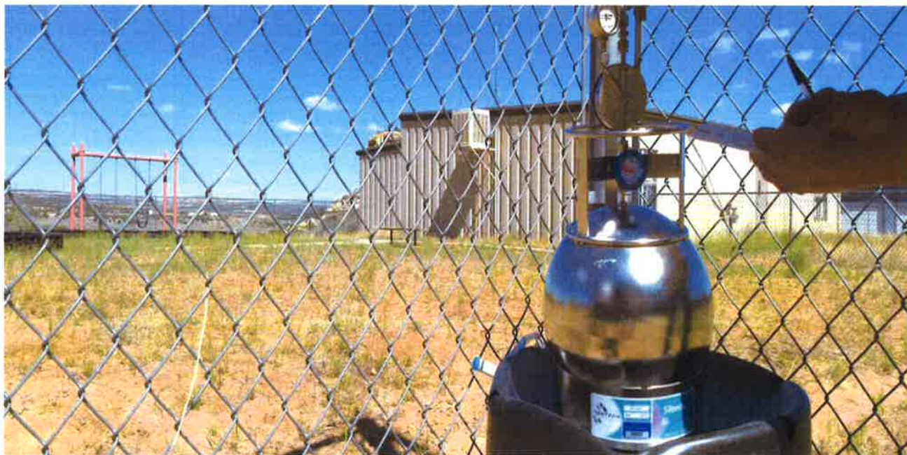
Figure 5: Summa Canister monitoring Volatile Organic Chemicals (VOCs) at Counselor Chapter House in May 2018.
