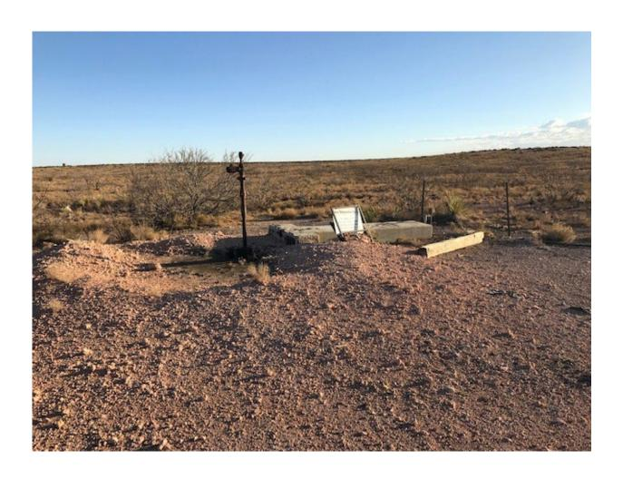
Mabel #005 (30-005-61908). Pump jack missing motor and other essential parts and no rods (3 photos).
