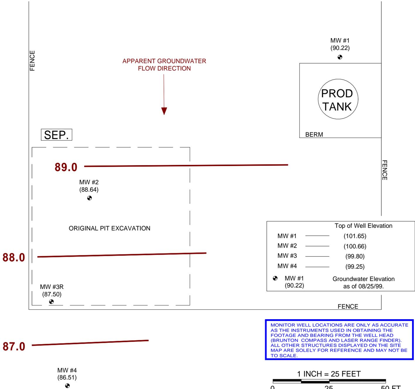
MONITOR WELL LOCATIONS ARE ONLY AS ACCURATE AS THE INSTRUMENTS USED IN OBTAINING THE FOOTAGE AND BEARING FROM THE WELL HEAD (BRUNTON COMPASS AND LASER RANGE FINDER). ALL OTHER STRUCTURES DISPLAYED ON THE SITE MAP ARE SOLELY FOR REFERENCE AND MAY NOT BE TO SCALE.
