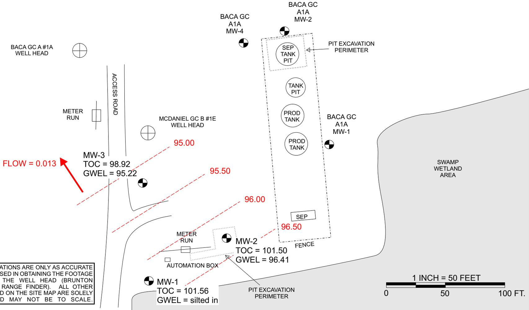
MONITORING WELL LOCATIONS ARE ONLY AS ACCURATE AS THE INSTRUMENTS USED IN OBTAINING THE FOOTAGE AND BEARING FROM THE WELL HEAD (BRUNTON COMPASS AND LASER RANGE FINDER). ALL OTHER STRUCTURES DISPLAYED ON THE SITE MAP ARE SOLELY FOR REFERENCE AND MAY NOT BE TO SCALE.
