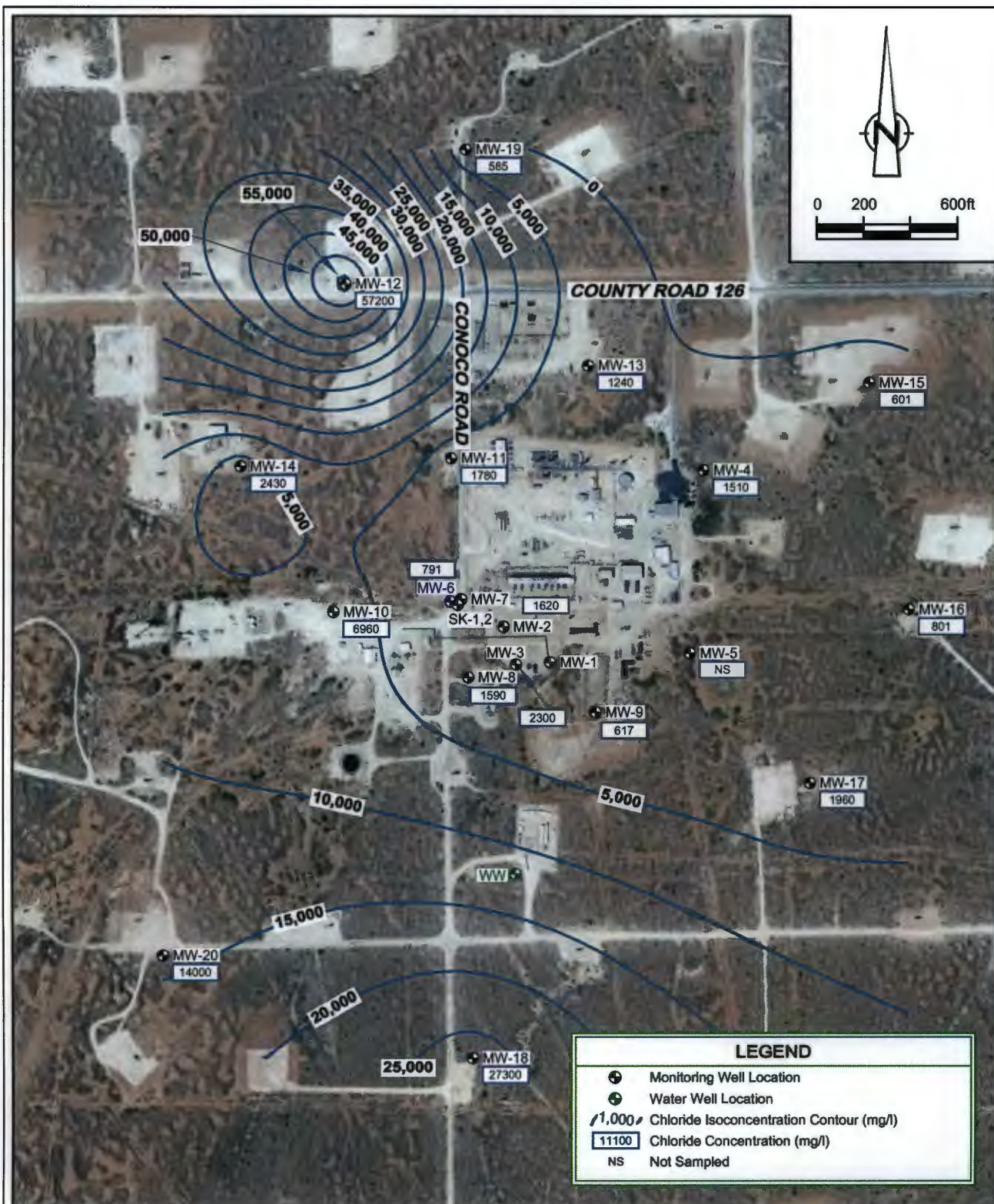
figure 7 CHLORIDE CONCENTRATION MAP -JULY 2012 MALJAMAR GAS PLANT LEA COUNTY, NEW MEXICO Phillips 66 Company
