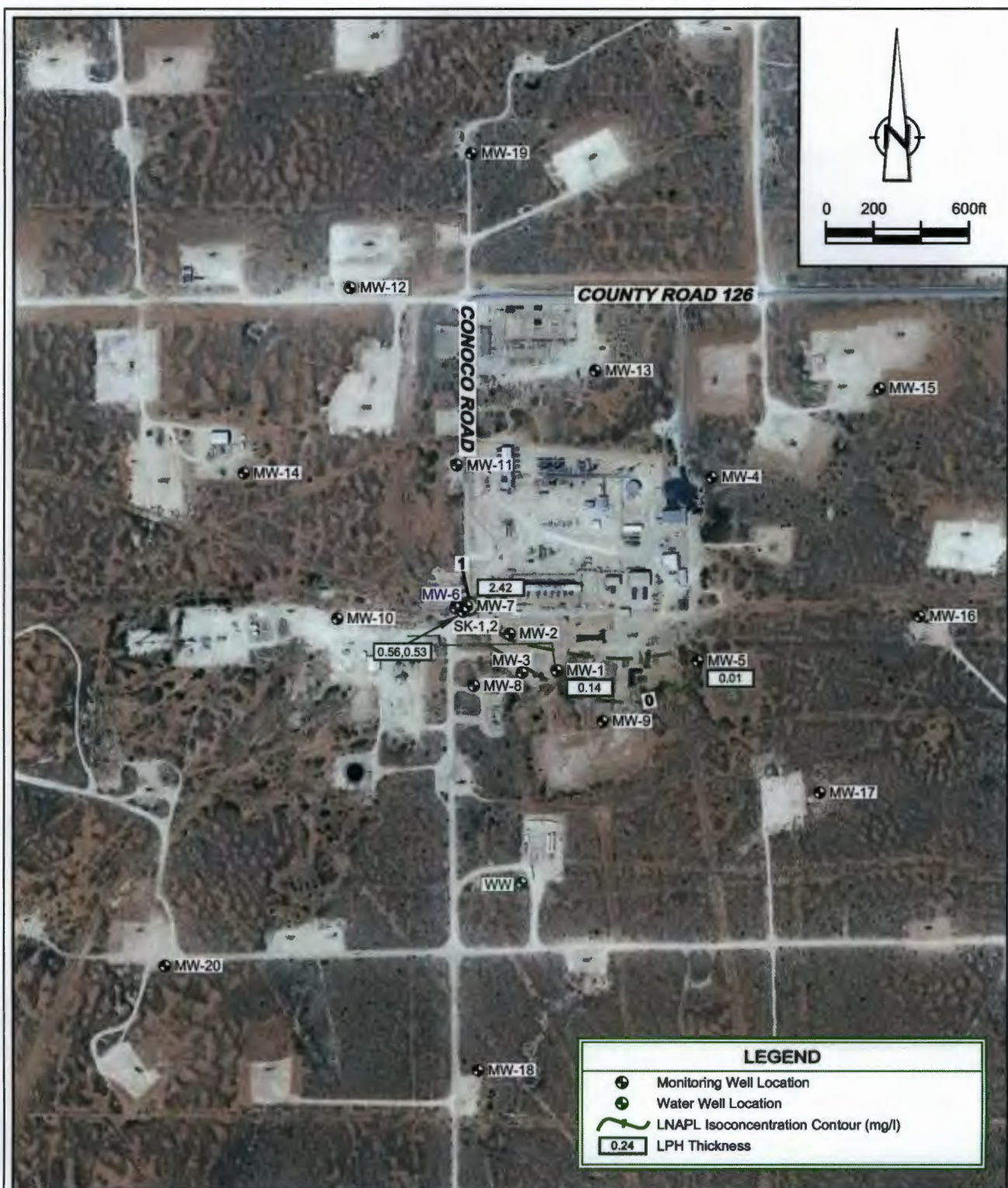
figure 5 LIQUID PHASE HYDROCARBON (LPH) THICKNESS CONTOUR MAP - JULY 2012 MALJAMAR GAS PLANT LEA COUNTY, NEW MEXICO Phillips 66 Company
