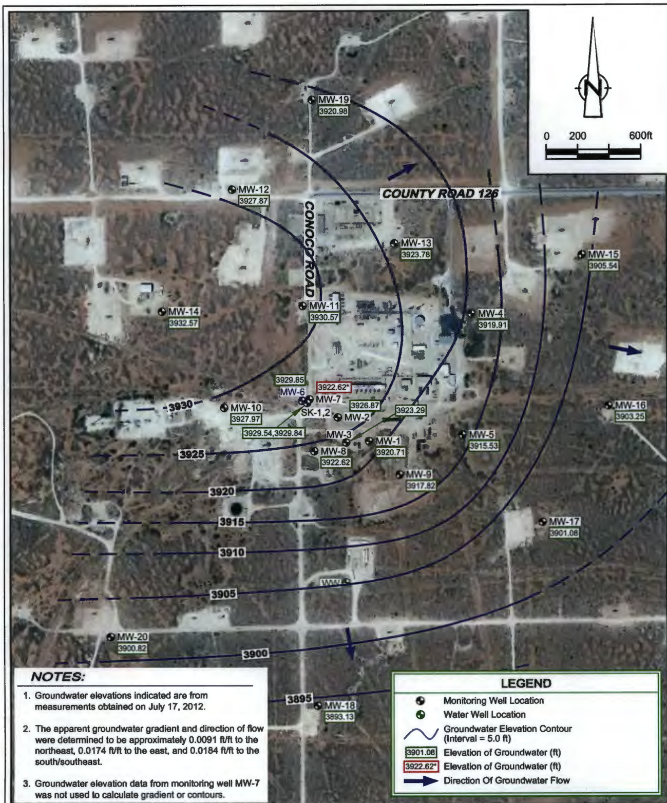
figure 3 GROUNDWATER GRADIENT MAP - JULY 2012 MALJAMAR GAS PLANT LEA COUNTY, NEW MEXICO Phillips 66 Company
