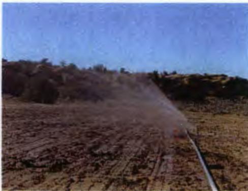
BP Americas Florence K5M showing produced water application
