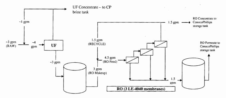
Figure 2, 2008 Pilot Equipment Flow Diagram
