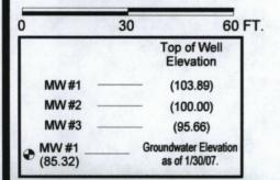
MONITOR WELL LOCATIONS ARE ONLY AS ACCURATE AS THE INSTRUMENTS USED IN OBTAINING THE FOOTAGE & BEARING FROM THE WELL HEAD (TAPE MEASURE, LASER RANGE FINDER, & BRUNTON COMPASS). ALL OTHER STRUCTURES DISPLAYED ON THIS MAP ARE SOLELY FOR REFERENCE AND MAY NOT BE TO SCALE.
