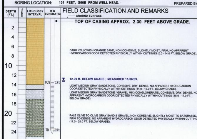
LIGHT MEDIUM GRAY SANDSTONE, COHESIVE, DRY, DENSE, NO APPARENT HYDROCARBON ODOR DETECTED PHYSICALLY WITHIN CUTTINGS (14.0 - 15.0 FT. BELOW GRADE). LIGHT MEDIUM GRAY SANDSTONE / GRAVEL MIX (CONGLOMERATE), COHESIVE, DRY, DENSE, NO APPARENT HYDROCARBON ODOR DETECTED PHYSICALLY WITHIN CUTTINGS (15.0 - 17.0 FT.
