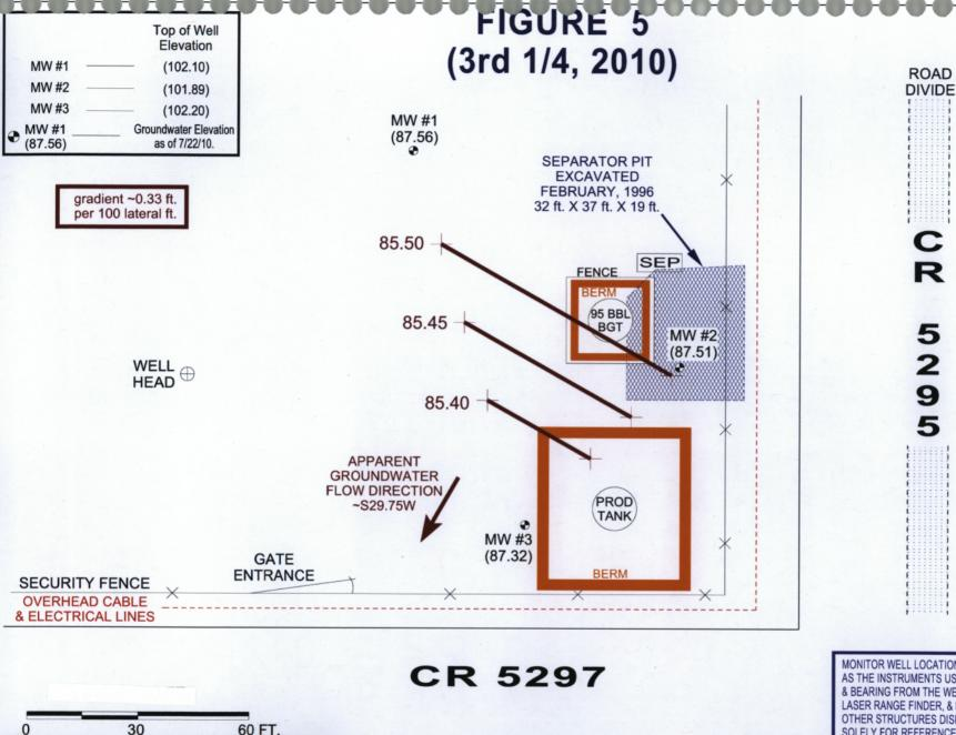
MONITOR WELL LOCATIONS ARE ONLY AS ACCURATE AS THE INSTRUMENTS USED IN OBTAINING THE FOOTAGE & BEARING FROM THE WELL HEAD (TAPE MEASURE, LASER RANGE FINDER, & BRUNTON COMPASS). ALL OTHER STRUCTURES DISPLAYED ON THIS MAP ARE SOLELY FOR REFERENCE AND MAY NOT BE TO SCALE.
