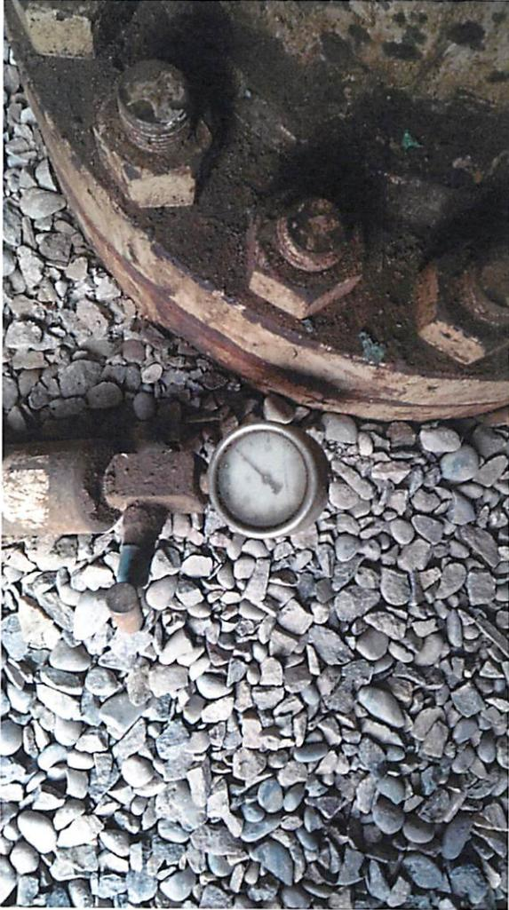
Bradenhead gauge at bottom of injection well
