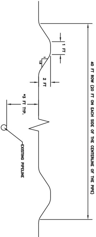
**Section E-E: 2 FOOT PIPELINE RIGHT OF WAY BERM**
