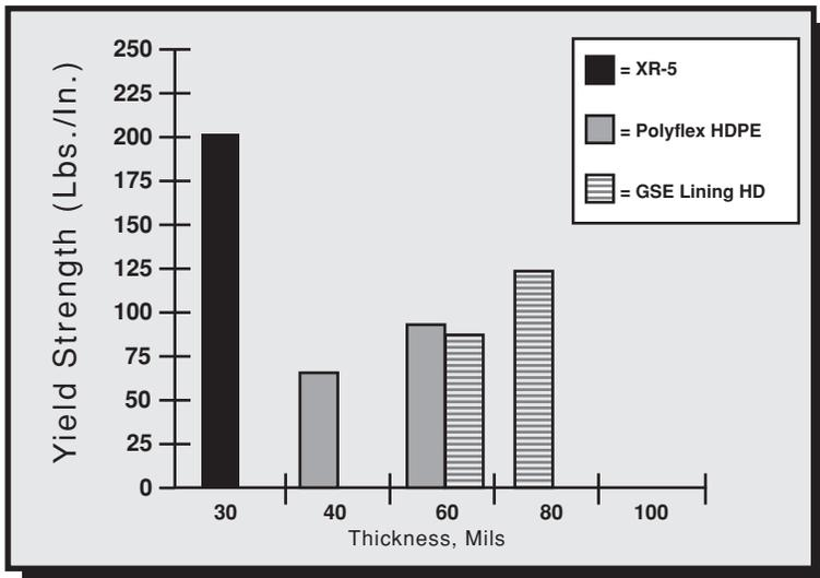
3. Strip tensile, ASTM D 751, 70°C\*
