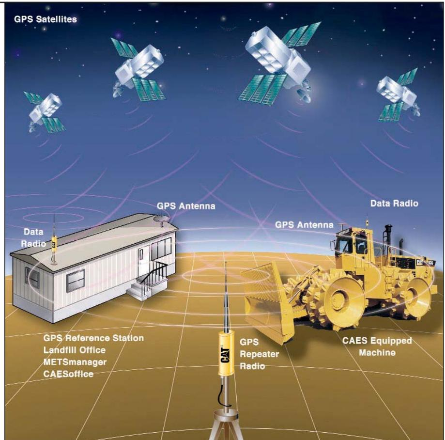
**CAESoffice™.** The powerful Caterpillar-designed CAESoffice software enables landfill management to monitor CAES-equipped machines and work progress throughout the site in near real-time. The data is stored in a database format for easy customized access, reporting and editing.
