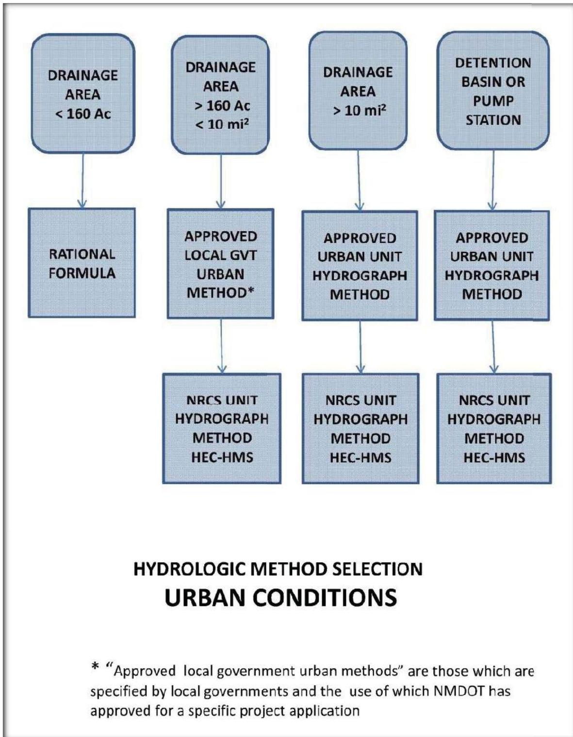
**Figure 401-2 Hydrologic Method Selection – Urban Conditions**
