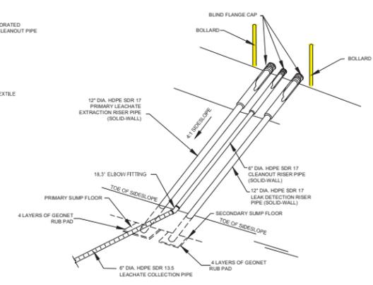
**B5 SUMP CLEANOUT/RISER CONFIGURATION SCHEMATIC**
