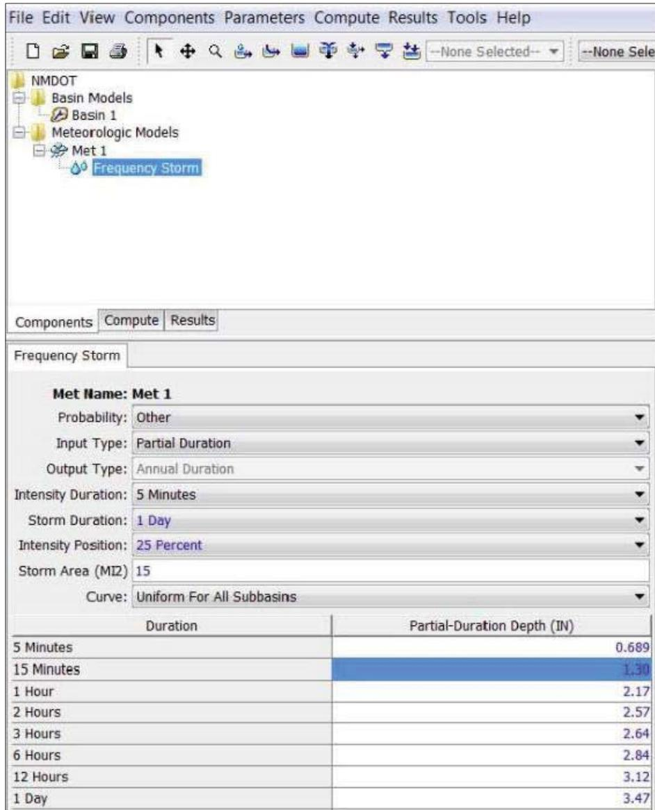
**Figure 405-3 Sample HEC-HMS Precipitation Input Table**
