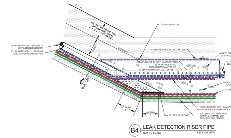
**B4 LEAK DETECTION RISER PIPE**
