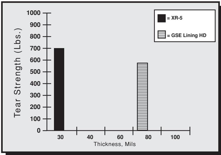
2. Graves Tear, ASTM D 624, Die C, 70°C\*
