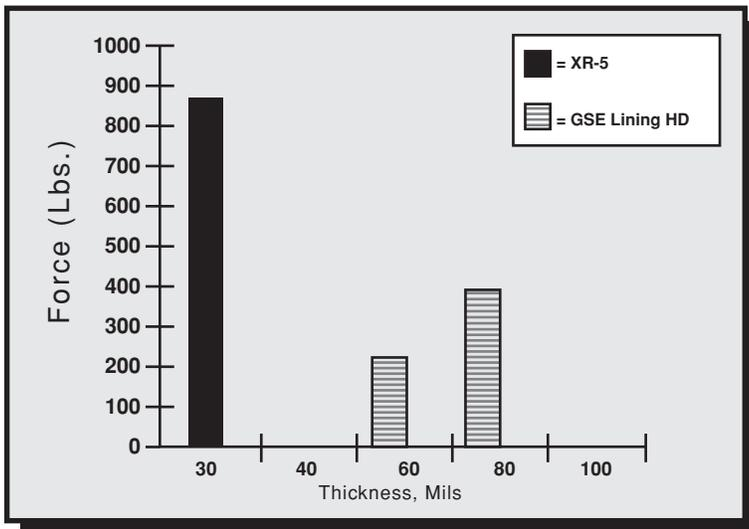
5. ASTM D 751 Ball Burst Puncture
