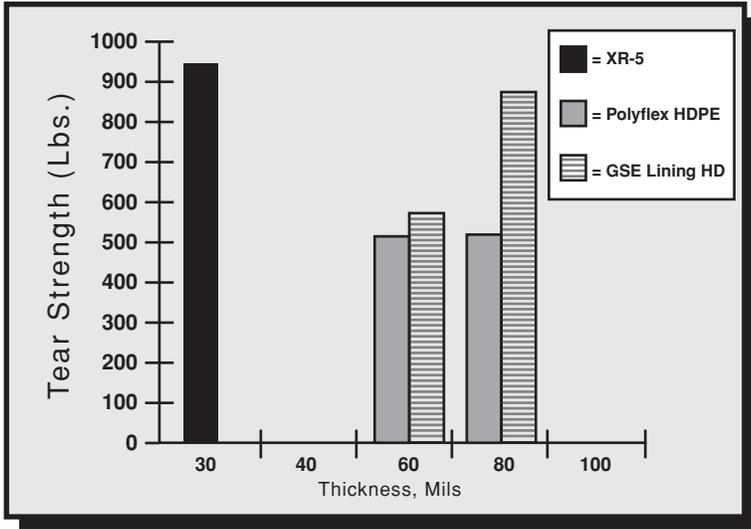
1. Graves Tear, ASTM D 624, Die C, Room Temperature\*
