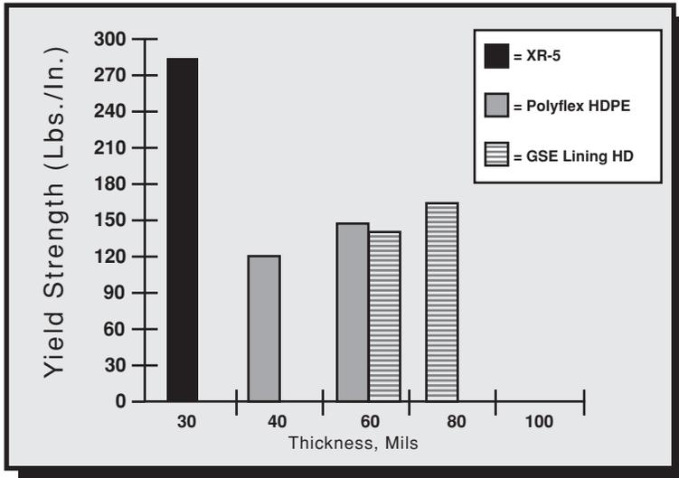
2. Strip Tensile, ASTM D 751, Room Temperature\*
