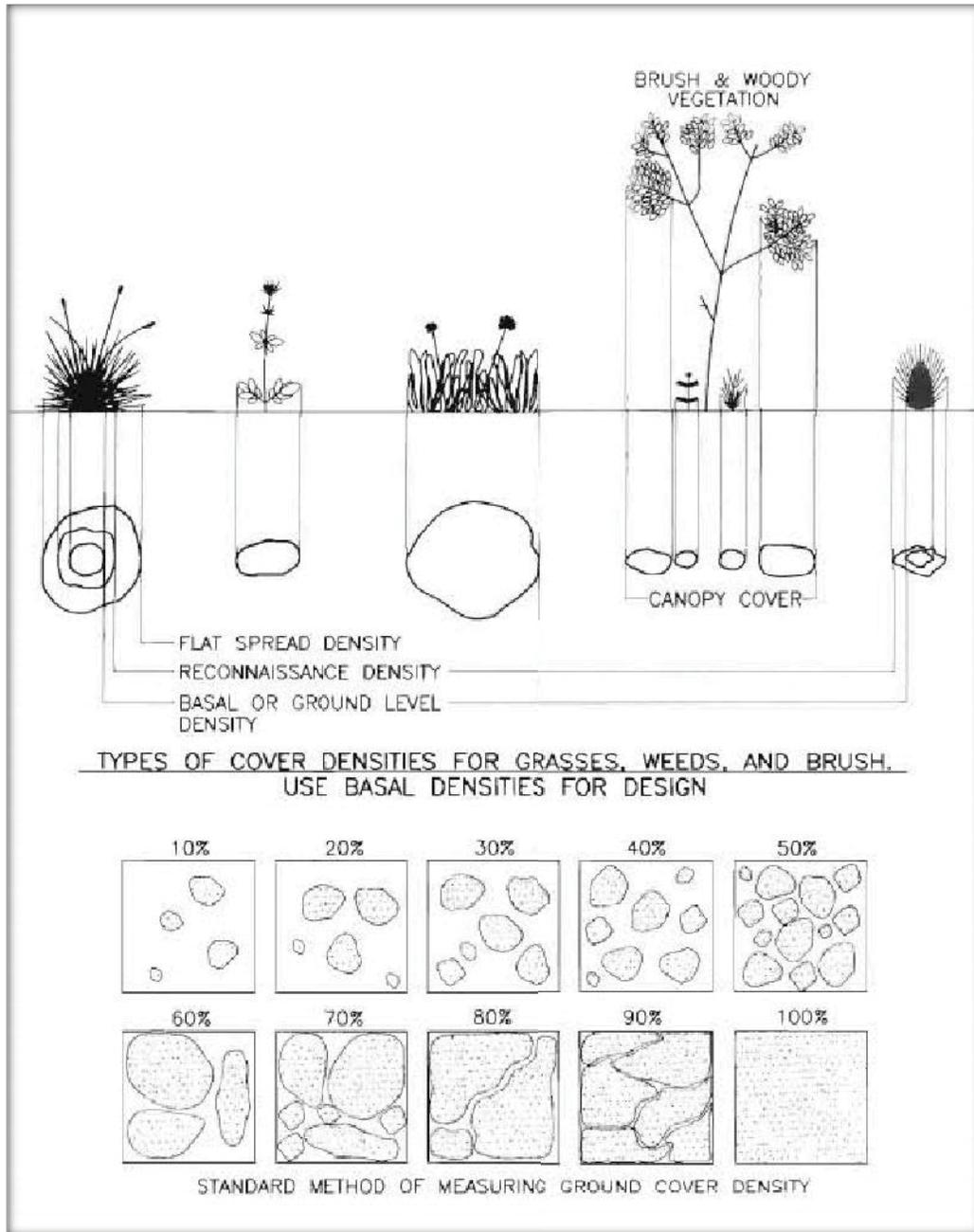
**Figure 402-6 Determining Soil-Cover Complex – Vegetative Density**
