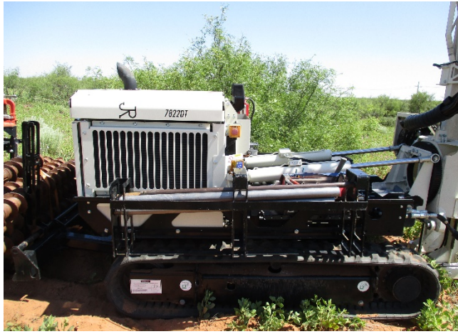
1. View of 7822DT Geoprobe rig used to advance soil borings.
