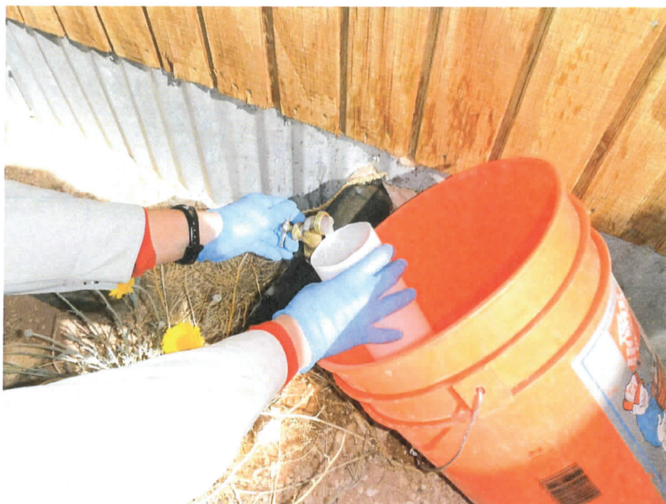
Photo 2 - Collection of sample from ICP-DHR-02 ("Tower") well. Previous to sampling, a hose was connected to spigot that discharged into a tank labeled "DO NOT USE THIS TANK".
