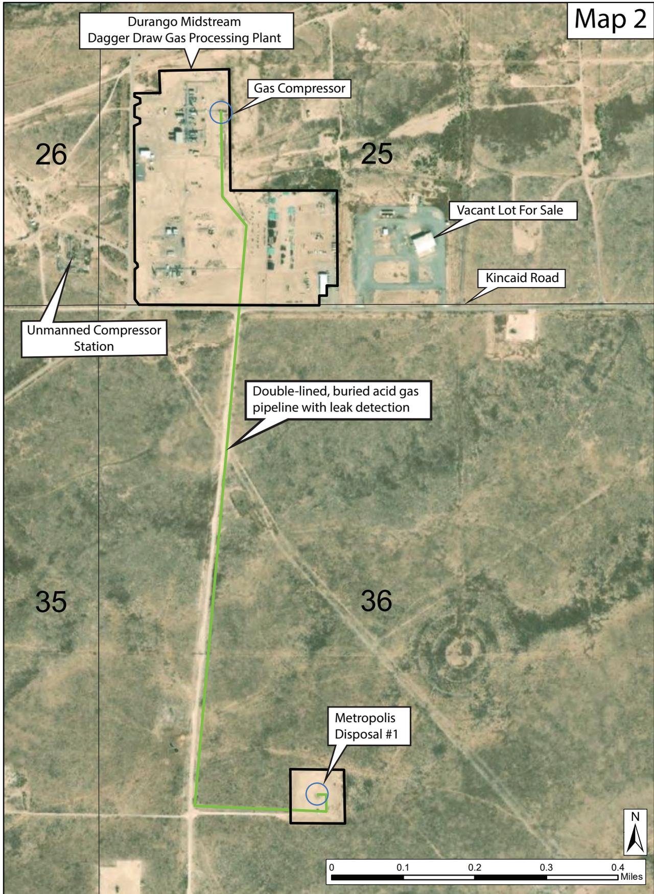
Map 2: General Diagram of Durango Dagger Draw Gas Plant and location of pipeline connecting the Plant with the Metropolis Disposal #1 Well. Please note that the former Agave Facility located immediately south of the Plant is inactive and unmanned.
