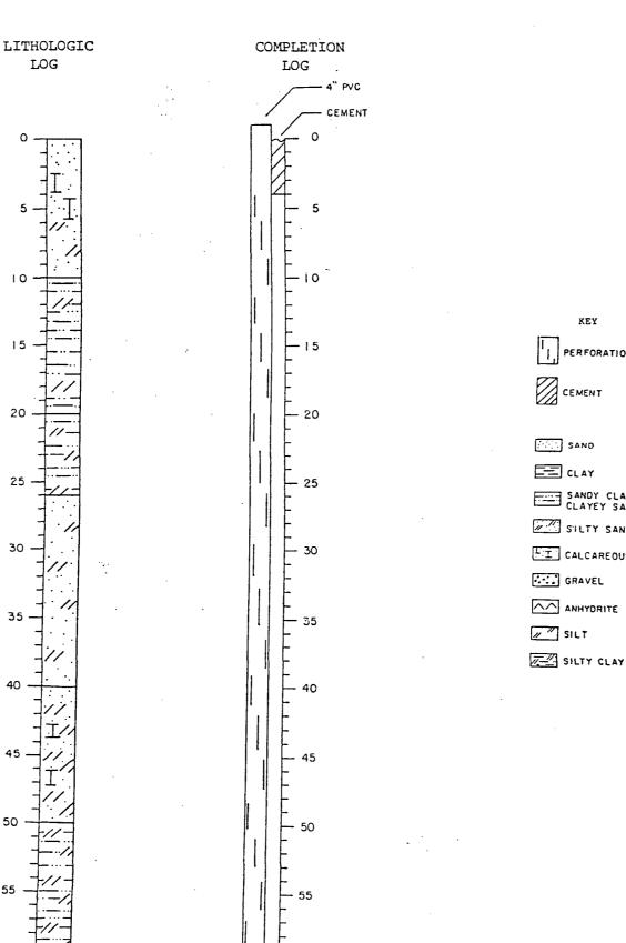
KEY PERFORATIONS SAND E CLAY E SANDY CLAY OR CLAYEY SAND STLTY SAND LI CALCAREOUS SAND GRAVEL ANHYDRITE
