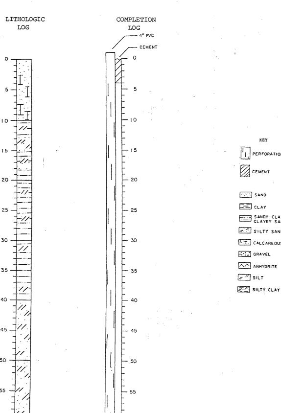
KEY PERFORATIONS SAND CLAY SANDY CLAY OR CLAYEY SAND SILTY SAND TI CALCAREOUS SAND GRAVEL
