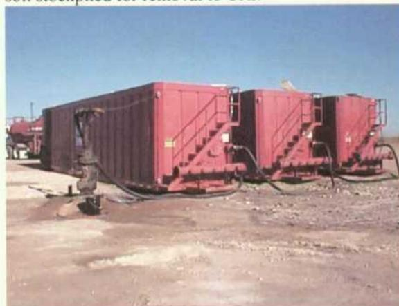
Photo 2: Temporary Produced water receiving system.
