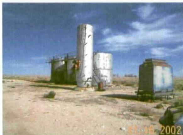
Photo 1. Treating plant is closing. The three tanks on site are part of a water station. The treater and other equipment is all that remains of the treating plant.
