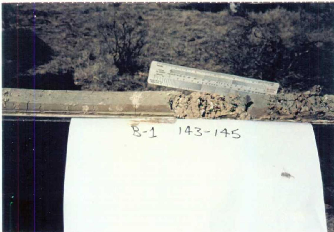
Photograph 4. Boring B-1 (MW-1), 143 -145 feet (02-03-98).
