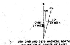
UTM GRID AND 1979 MAGNETIC NORTH DECLINATION AT CENTER OF SHEET
