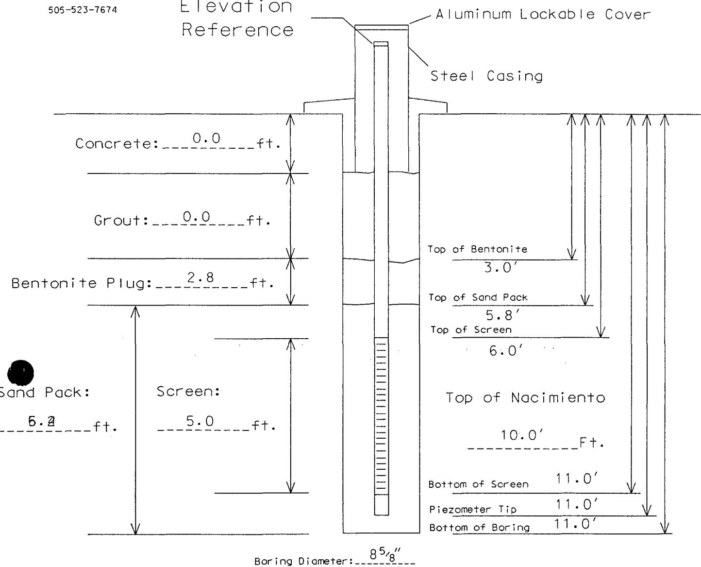
Sand Type: 10-20 SilicaBollards, Type/Size: NABentonite:  $\frac{3}{8}$ " ChipsScreen Type/Size: 2" PVC Sch. 40, 0.010" SlottedCement/Grout: NARiser Type/Size: 2" PVC Sch. 40Water: PotableLocking Expandable Casing Plug? Yes Site Northing: TBS
