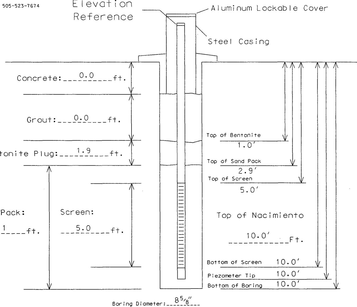
Sand Type: 10-20 SilicaBollards, Type/Size: NABentonite: 3/8" ChipsScreen Type/Size: 2" PVC Sch. 40, 0.010" SlottedCement/Grout: NARiser Type/Size: 2" PVC Sch. 40Water: PotableLocking Expandable Casing Plug? Yes Site Northing: TBS
