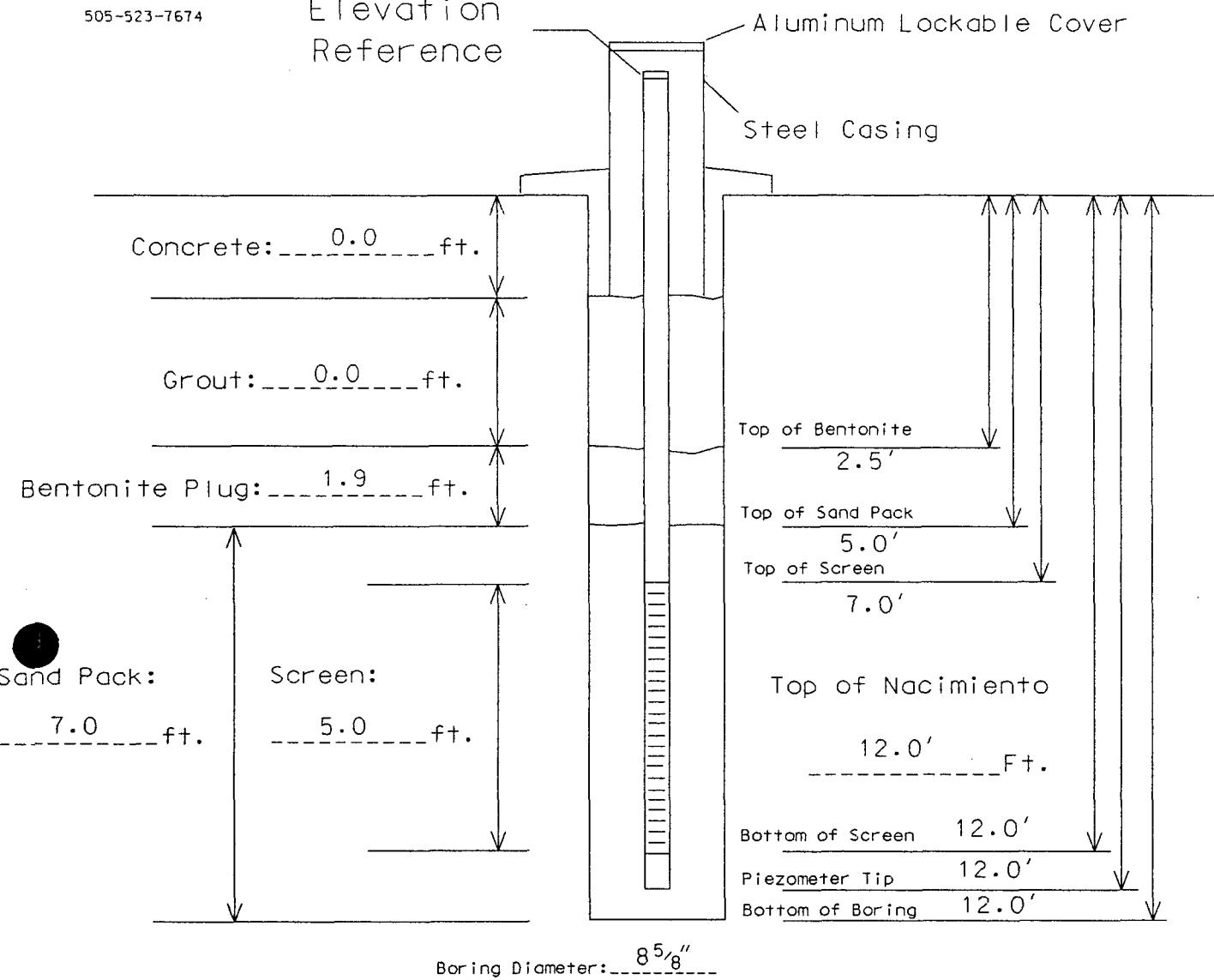
Boring Diameter: 8 5/8"Sand Type: 10-20 SilicaBollards, Type/Size: NABentonite: 3/8" ChipsScreen Type/Size: 2" PVC Sch. 40, 0.010" SlottedCement/Grout: NARiser Type/Size: 2" PVC Sch. 40Water: PotableLocking Expandable Casing Plug? Yes Site Northing: TBS
