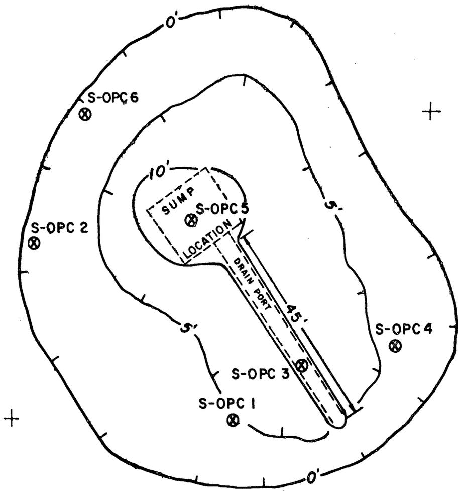
NOTE: FIGURE PORTRAYS STATUS OF EXCAVATION FOLLOWING INITIAL REMOVAL OF FIBERGLASS LINER AND SUMP SYSTEM.
