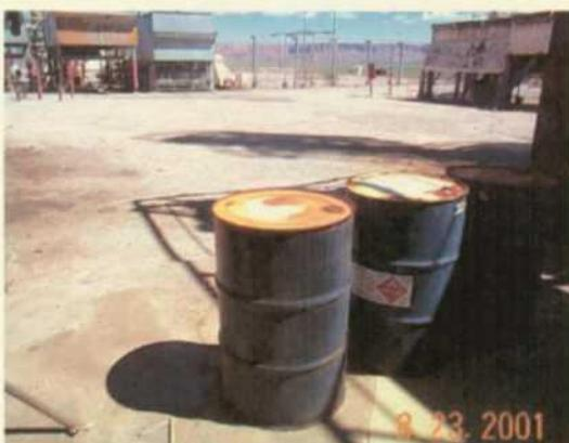
Pic # 3- Methanol drums in FCC area-need proper containment.
