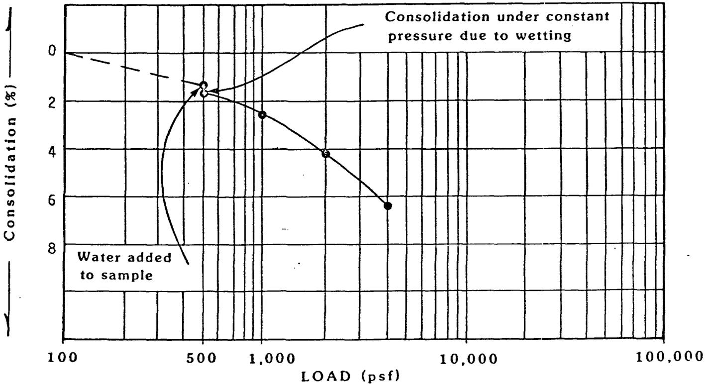
Sample of very clayey SAND from test hole 2 at depth 6 feet.
