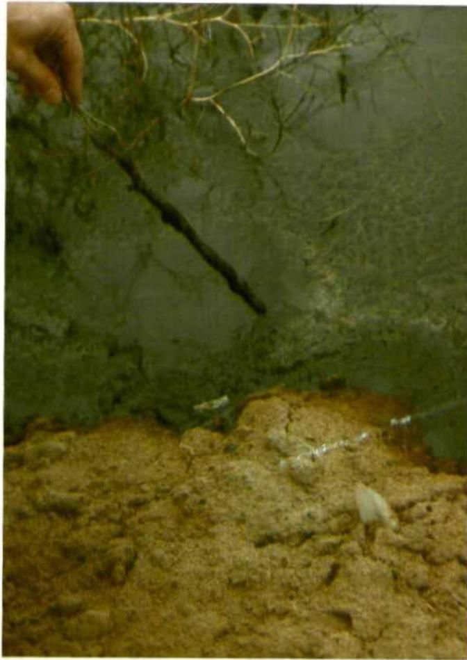
Figure 2-5 Photograph of edge of impoundment at East Lee Acres showing petroleum product sludge floating on surface 3/12/85.
