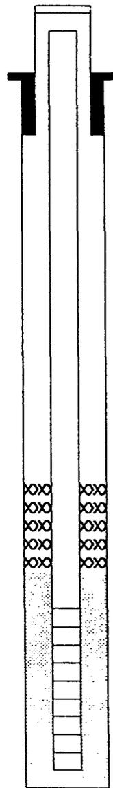
Comments: WATER LEVEL AT 17.5 AFTER INSTALLATION. 7.5 BAGS OF SAND, 1 1/2 BUCKETS OF SAND
