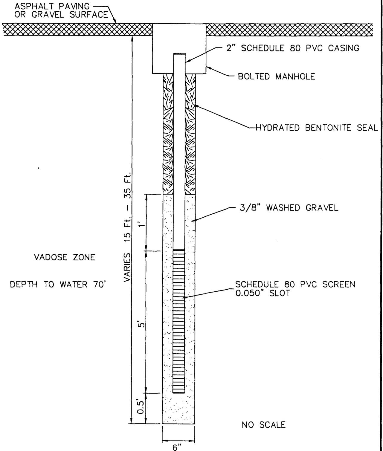
FIGURE 2-2: TYPICAL EXTRACTION WELL FOR SVE PILOT TEST, DOWELL SCHLUMBERGER INCORPORATED, HOBBS, NEW MEXICO
