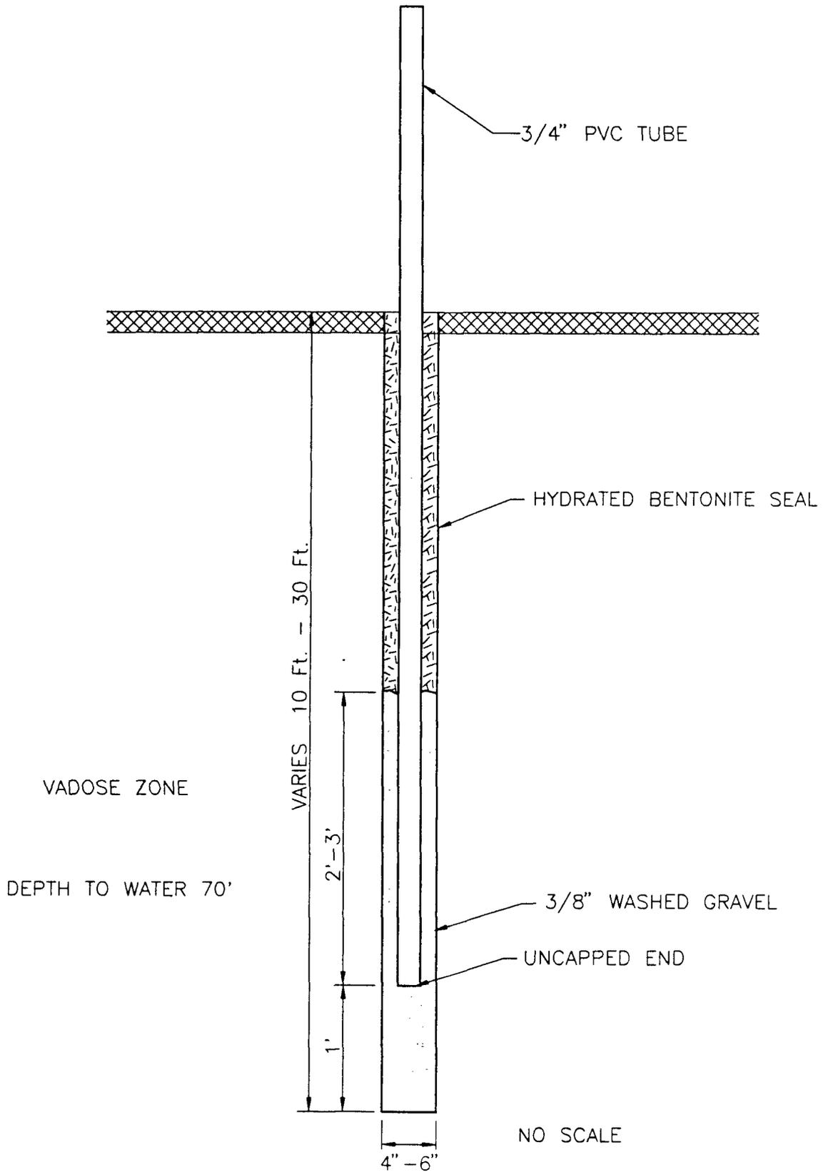
FIGURE 2-3: TYPICAL PIEZOMETER FOR PRESSURE MONITORING DURING SVE PILOT TEST, DOWELL SCHLUMBERGER INCORPORATED, HOBBS, NEW MEXICO
