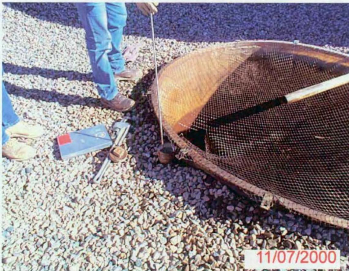
Picture #3- Leak Detector has fluids with oil and water observed on dip-stick.
