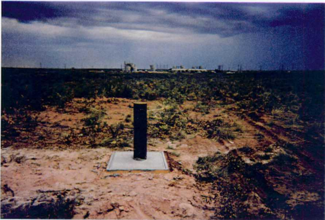
Completed monitor well ACW-12
