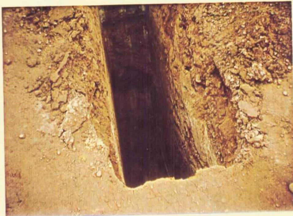
28. View into exploratory trench excavated south of the gateway. Note absence of hydrocarbon stain on sidewalls of trench.
