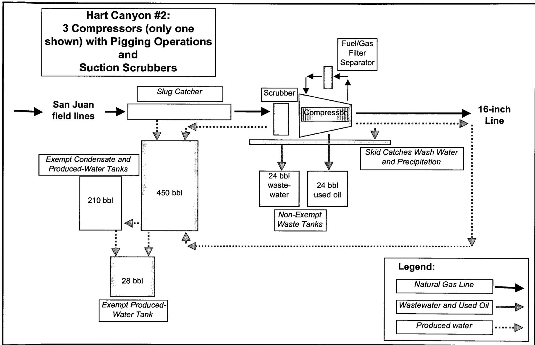
**Plate 1: Process Map of Hart #2 Compressor Station**
